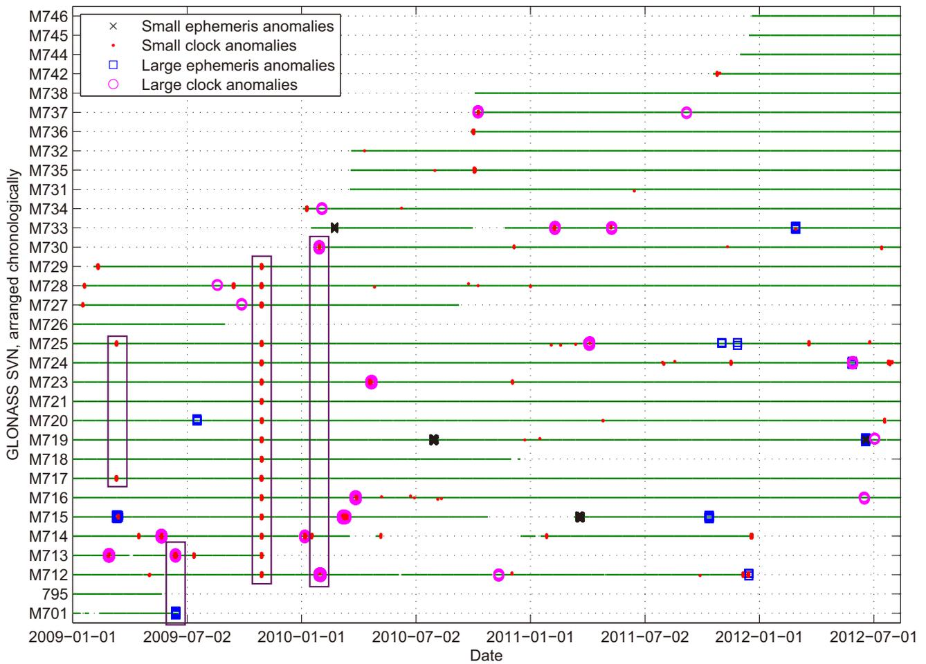
**Figure 3.** Identified GLONASS SIS anomalies between Jan 1, 2009 and Aug 11, 2012. The horizontal green lines depict the periods when the satellites were active (not necessarily healthy). The purple rectangles indicate simultaneous multiple anomalies, including a constellation-wide event on Oct 28, 2009.
