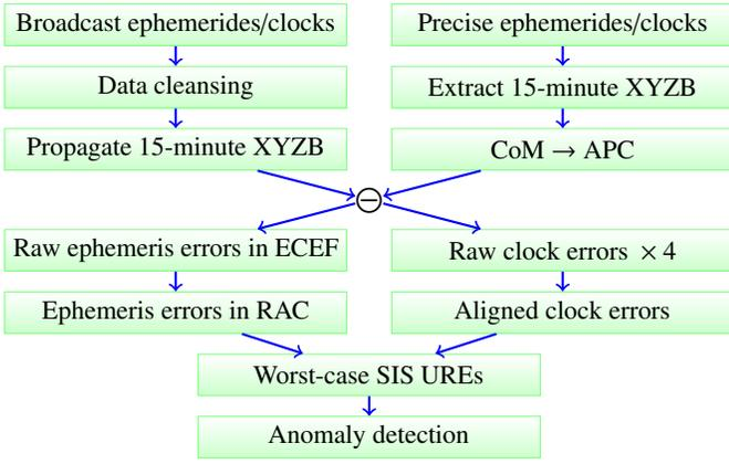
**Figure 2.** Framework of the whole process. XYZB values refer to the coordinates of satellite position in ECEF and satellite clock bias. RAC refer to the radial, alongtrack, and crosstrack-based satellite centered coordinate system.
