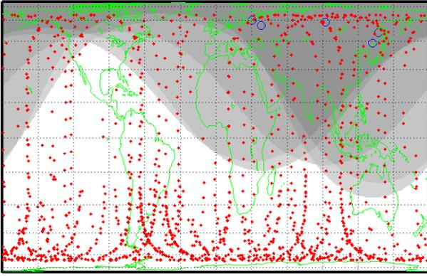
**Figure 7.** Ground tracks (denoted by red dots) of anomalous GLONASS satellites since Jan 2010. The blue circles represent the five existing GLONASS monitor stations [29]. The shaded areas indicate the tracking coverage of these monitor stations.
