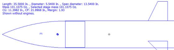
**Figure 5:** Aerodynamic Shell Design and RockSim simulation results
