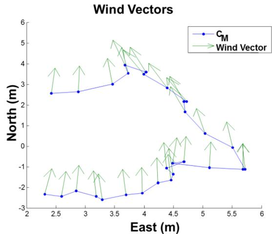
**Figure 14:** Quiver plot of wind velocities and heading on the payload center of mass
