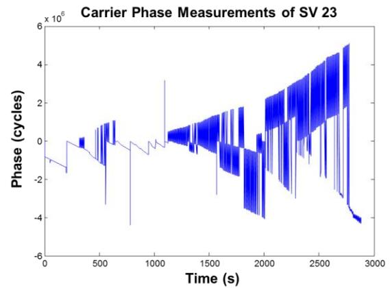
**Figure 9:** Multiple cycle slips occurred due to the erratic dynamics of the aerostat.
