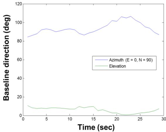
**Figure 12:** Baseline direction for sensing payload attitude determination
