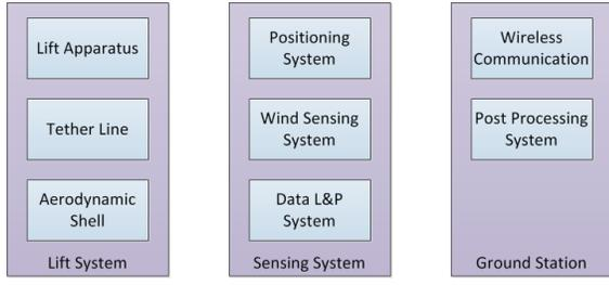
**Figure 3.** System Architecture of GPS-based Wind Sensing System
