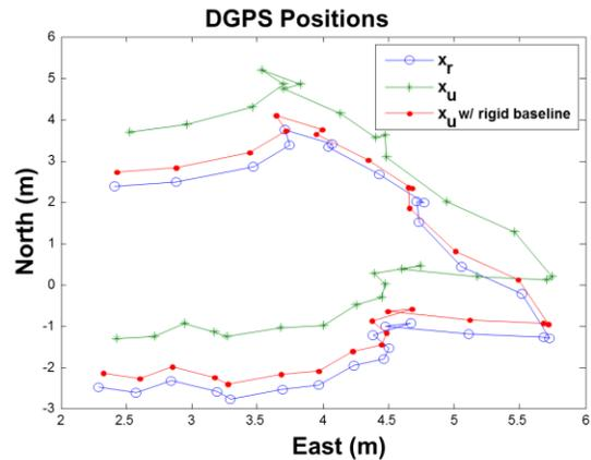
**Figure 10:** DGPS Positions of the user and reference receiver antennae on-board the sensing payload.
