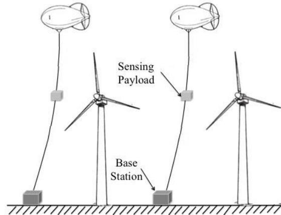
**Figure 1.** Concept depiction of wind sensing system in operation
