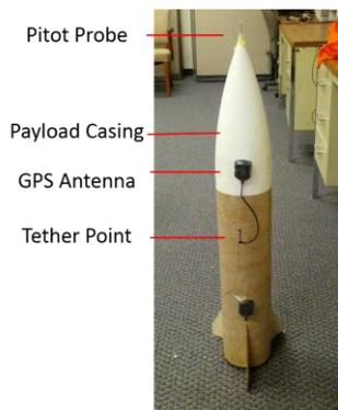
**Figure 6:** Payload Sensing System
