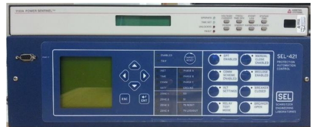
Figure 3: Two phasor measurement units from the TCIPG testbed at University of Illinois Urbana-Champaign.
