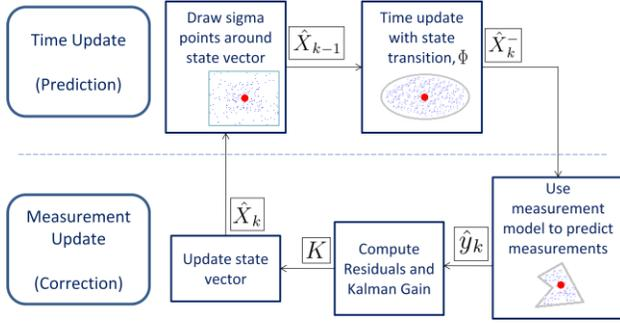
Figure. 4. The unscented Kalman filter (UKF). Consists of the Time update and Measurement update steps. Time update: we use the state transition matrix  $\Phi$  (Eq. 5) to propagate the states. Measurement update: we use the measurement model to predict measurements, compute the Kalman gain and update the states.
