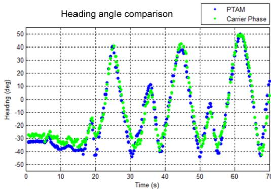
Figure 10. Comparison between the heading estimates obtained from PTAM (blue) and from the GPS carrier phase measurements (green). The heading estimates from the carrier phase measurements accurately match the heading estimates from PTAM.
