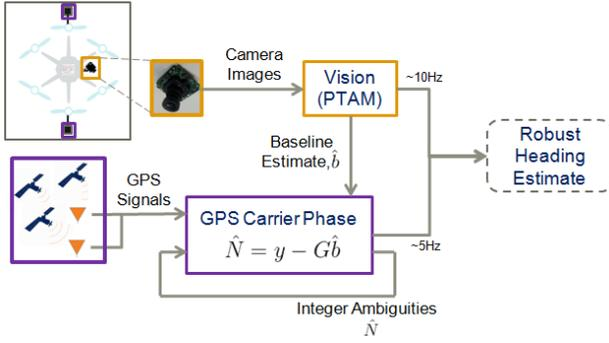
Figure. 3. Tightly-coupled initialization procedure to resolve carrier phase integer ambiguities. Once the ambiguities are resolved we obtain heading information from the GPS receivers, in addition to the vision algorithm.
