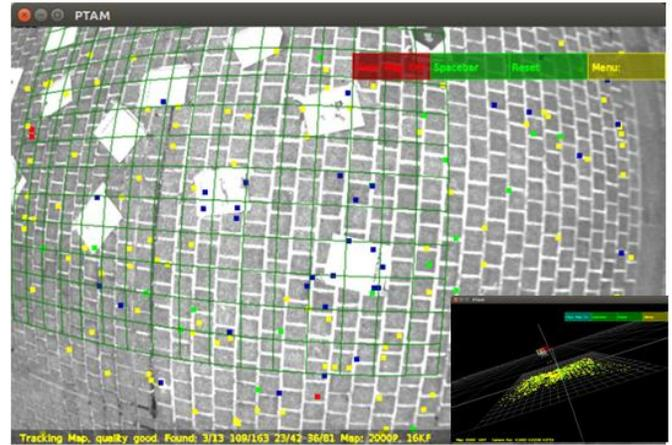
Figure 1. Parallel Tracking and Mapping (PTAM). Algorithm tracks features across images and re-projects them on a point cloud to estimate the cameras pose (bottom right).
