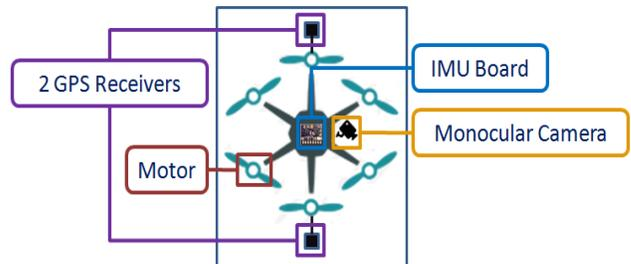
Figure 2. Components layout. Information sources for navigation: 2 GPS receivers, Monocular camera, IMU board and motors.
