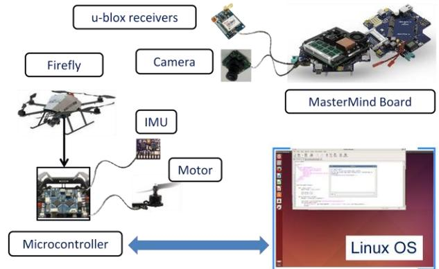
Figure. 8. Hardware components used for collecting flight data. The Mastermind with the Linux OS records all the incoming information used later on for post-processing.
