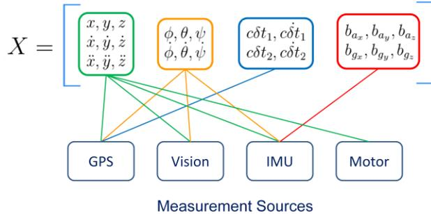
Figure. 6. Correction model block diagram. The four measurement sources affect different states in the Measurement update step of the UKF.
