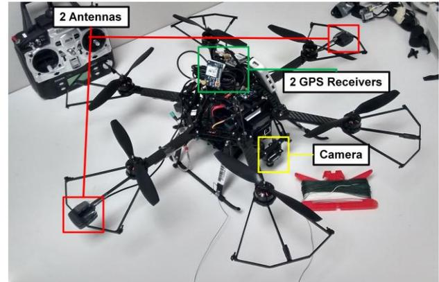
Figure. 7. Ascending Technologies Firefly hexacopter setup used for flight experiments. Two GPS antennas are mounted on opposite arms along with a downward facing camera.
