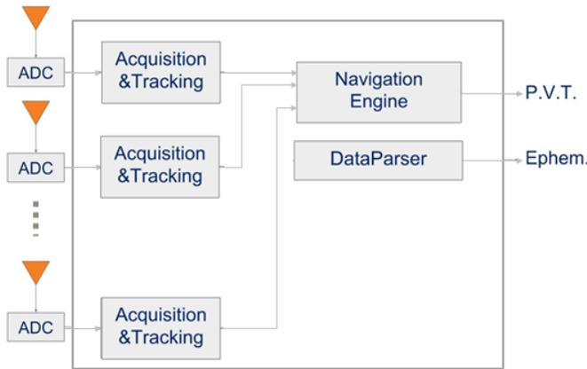
**Figure 1.** Approach overview. Multiple antennas track the signals from visible GPS satellites. These signals are sent to the respective receivers. Each receiver then applies acquisition and tracking algorithms to generate measurements like the pseudorange and the carrier phase. Finally the pseudorange measurements from all the receivers are then used in an extended Kalman filter, which estimates the position of the quadrotor.
