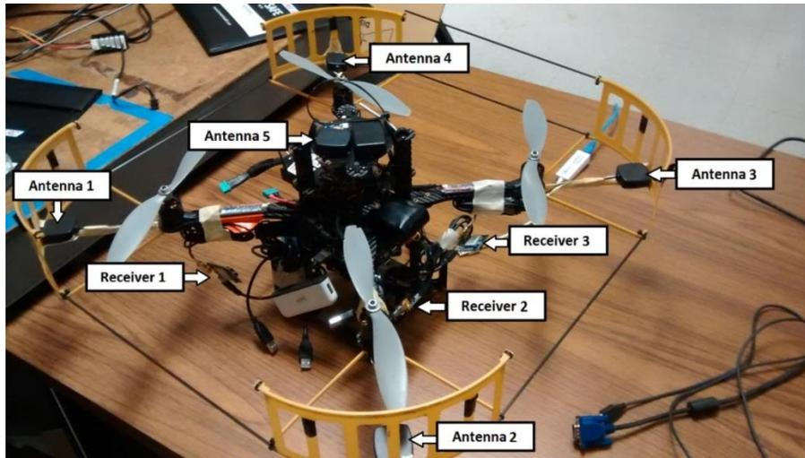
**Figure 2.** The AscTec Pelican labelled with the visible u-blox receivers and antennae placed on it. There is one receiver on each arm of the Pelican, and one at the center.
