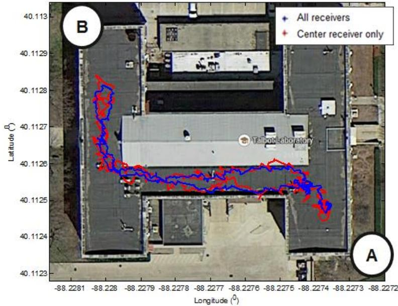
**Figure 5.** 2D trajectory of the Pelican on the Talbot Lab roof. It was moved from Point A to Point B, and then back to Point A. The multiple-receiver solution looks more accurate and is less scattered compared to the solution from the center receiver only.
