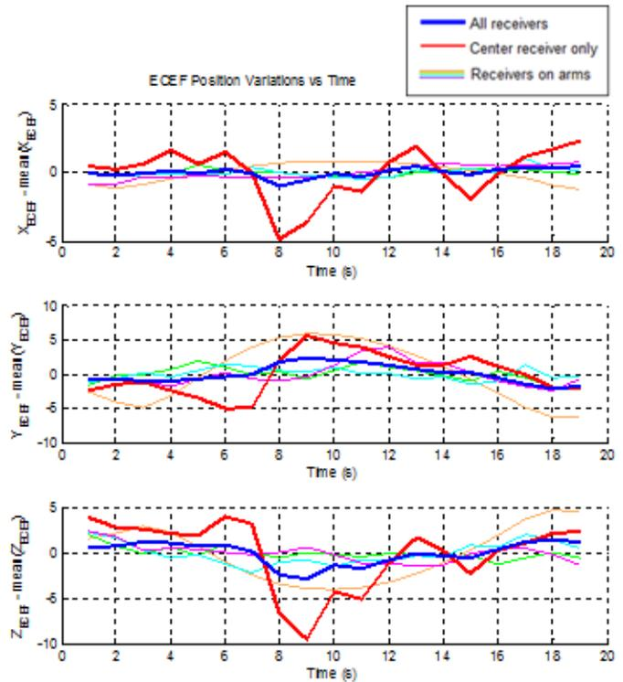
**Figure 4.** Variation in the position estimates while losing satellite ID 16 from view. There is a sharp jump in the estimates using only the center receiver, but the multiple-receiver solution is more robust to such a change.
