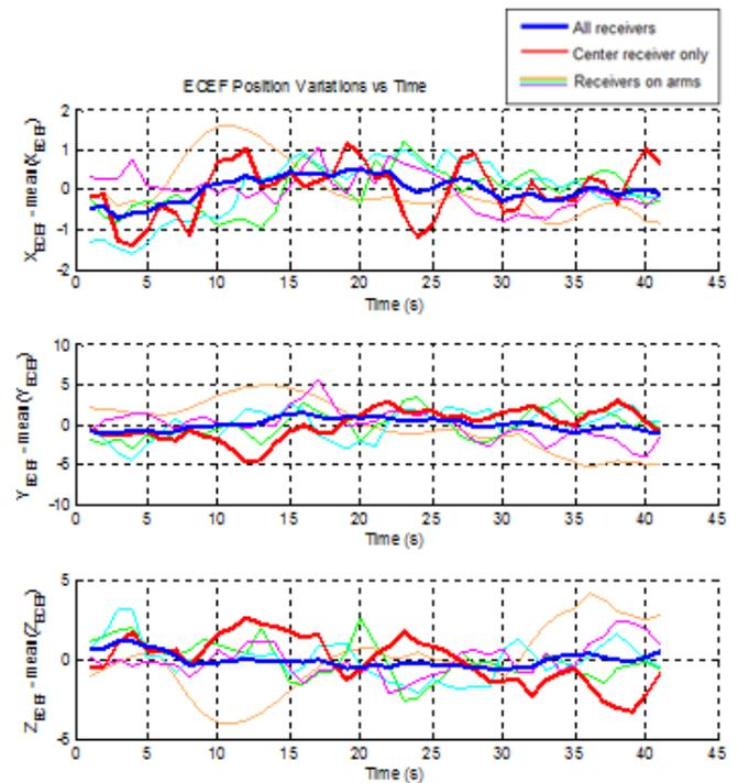
**Figure 3.** Variations in the position estimates of the stationary Pelican. The standard deviations using multiple-receivers are: [0.3227 0.7333 0.4536] meters in the ECEF x, y and z co-ordinates respectively. Using only the center receiver, we get standard deviations: [0.6780 1.8482 1.5240] meters.
