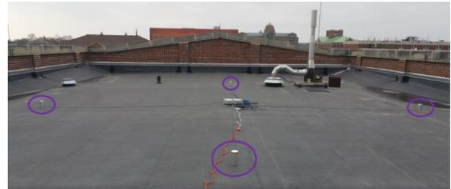
Figure 6: The antennas are placed at an approximately 10m radius.
