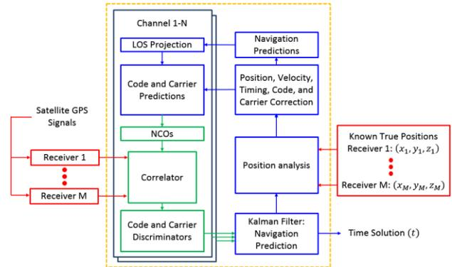
Figure 4: Multi-Receiver PIA Vector Tracking Loop
