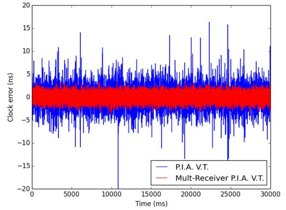
Figure 9: Time errors when 8dB of additional noise is added. Scalar tracking has stopped working.
