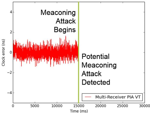
Figure 11: Time errors during a simulated meaconing attack with a 100m separation between the spoofer and the PMU GPS receivers.
