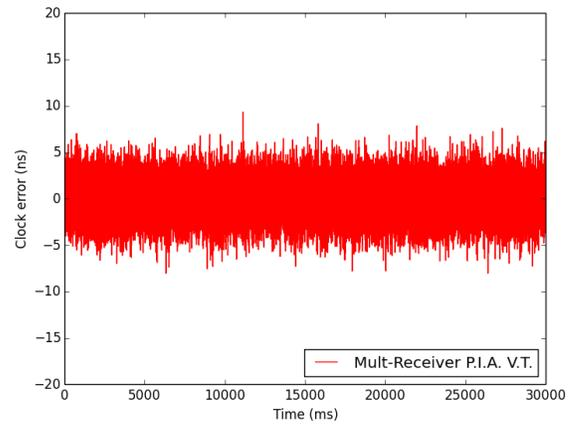
Figure 10: Time errors when 11dB of additional noise is added. Scalar and single-receiver PIA vector tracking have both stopped tracking.
