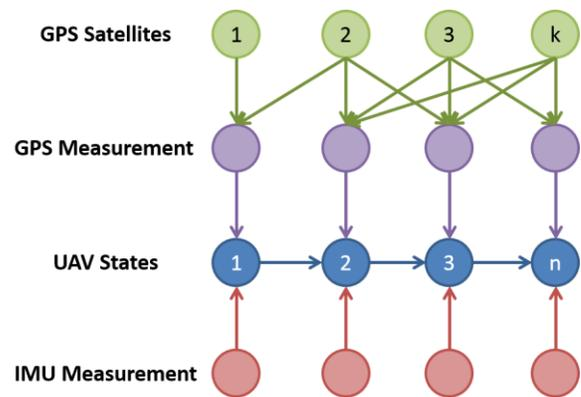
Figure 1: Visualization of GPS Probabilistic Graph
