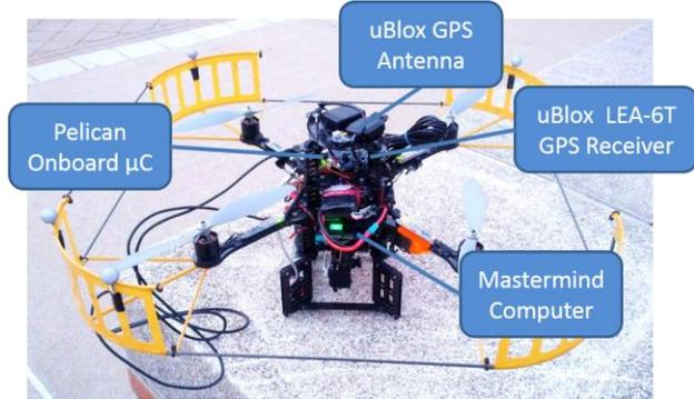
**Figure 2:** Experimental setup of an Asctec Pelican. It is equipped with an onboard IMU and an additional u-blox LEA-6T GPS receiver.
