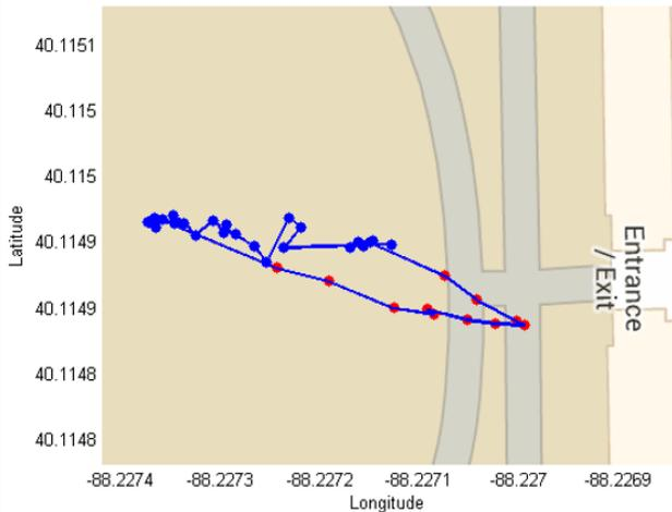
**Figure 7:** GPS navigation solution with a 10 s gap in satellite visibility
