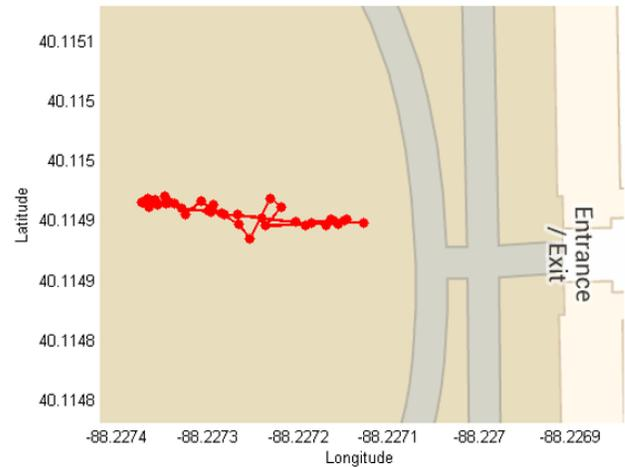
**Figure 4:** GPS only positioning of a UAV's trajectory.
