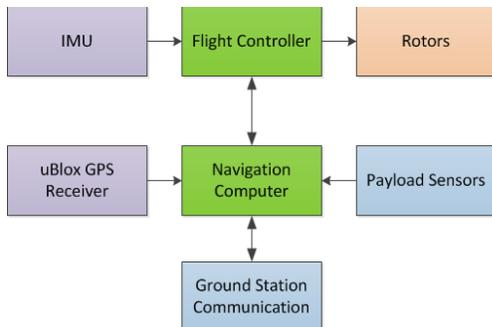
**Figure 3:** Command and Data Handling Diagram for the Asctec Pelican equipped with navigation equipment.
