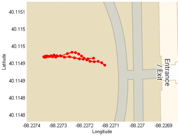
**Figure 6:** GPS with PGM estimated positioning of a UAV's Trajectory.
