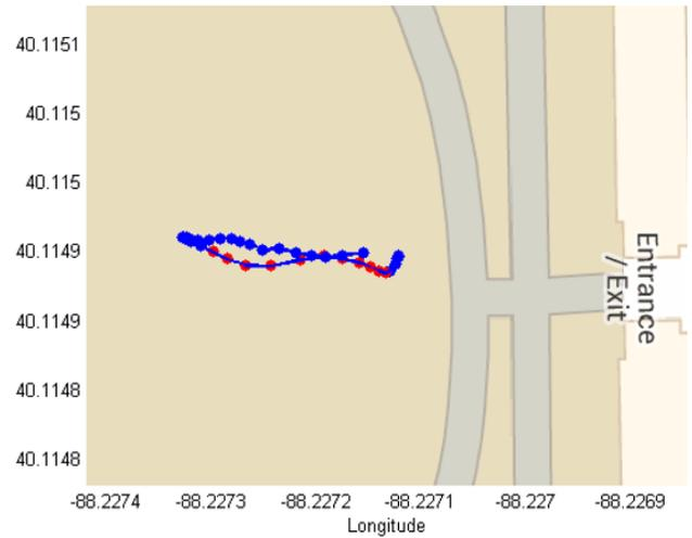
**Figure 8:** PGM improved GPS navigation solution with a 10 s gap in satellite visibility
