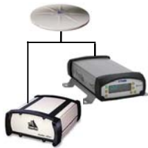
Figure 6. Commercial receivers setup in the GPS lab at Stanford, CA. The incoming signal received by a commercial patch antenna is split into two paths, one connecting to a commercial multi-band multi-constellation GNSS receiver, the other connecting to a GPS L1 only receiver.
