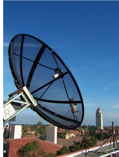
Fig. 3. The 1.8-meter parabolic antenna of the Stanford GNSS Monitoring Station, Stanford, California
