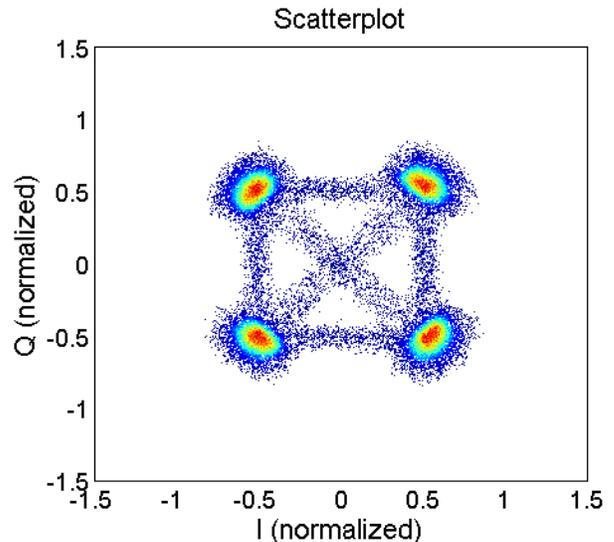
**Figure 5 Scatter plot of GLONASS-K1 L3 showing the IQ signal constellation histogram**
