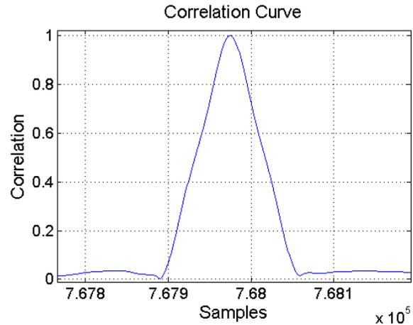
**Figure 10 Exemplary correlation function – cross correlation of theoretical code with samples of data channel**
