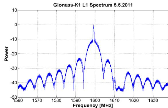
Figure 2 Normalized spectrum of GLONASS-K1 L1 signal recorded at maximum elevation at 05-05-2011
