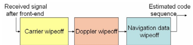
Figure 14. E5 code sequence demodulation diagram
