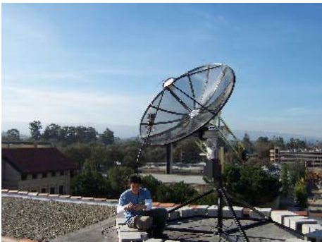
Figure 2. Stanford GNSS Monitor System, 1.8m dish
