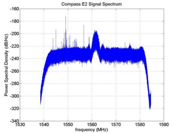
Figure 4. Unaveraged spectrum of Compass-M1 E2
