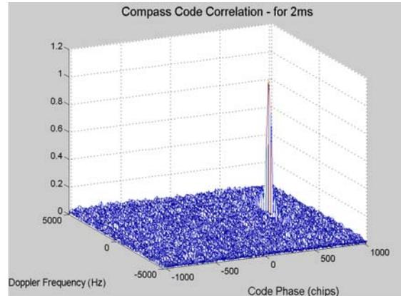
Figure 12. Acquisition plot of Compass-M1 E2 I-channel
