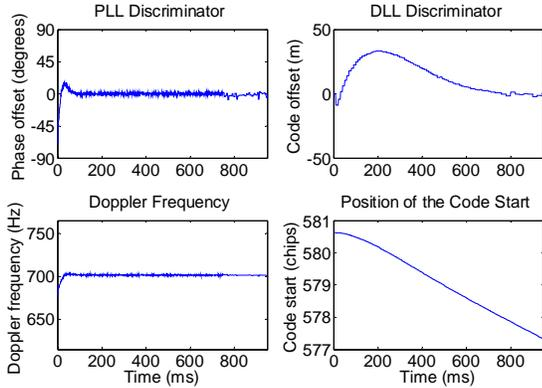
Figure 13. Tracking results of Compass-M1 E2 I-channel
