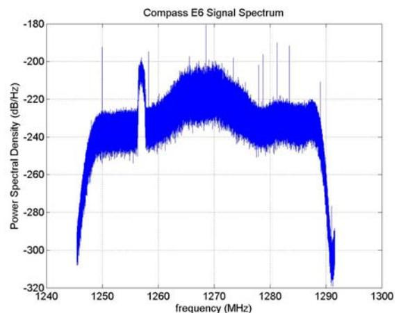
Figure 6. Unaveraged Spectrum of Compass-M1 E6
