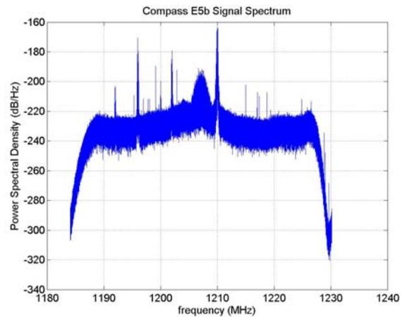
Figure 5. Unaveraged spectrum of Compass-M1 E5b
