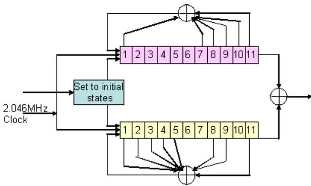
Figure 11. Code generator schematic of the Compass E2 I-channel signal
