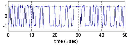
Figure 10. First 50 microseconds of the Compass E2 I-channel PRN code
