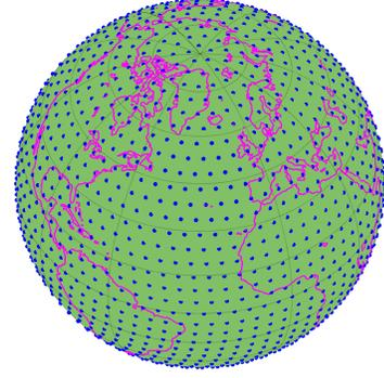
Fig. 6. DOP values are computed for 1807 points nearly evenly distributed on the Earth. The spherical distance between any two neighbor points is roughly  $5^\circ$ .
