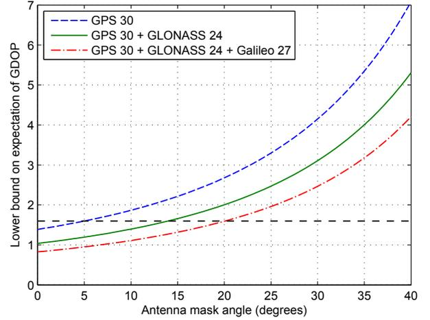
Fig. 4. Lower bound on expectation of GDOP calculated using (27) for one constellation comprised of 30 satellites, two constellations comprised of 54 satellites, and three constellations comprised of 84 satellites.
