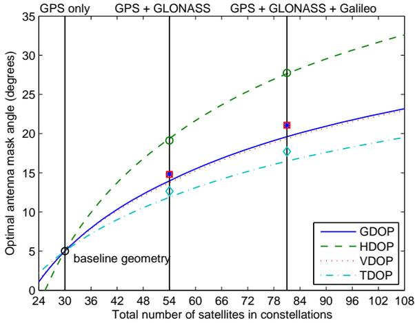
Fig. 7. Comparison between theoretical and numerical results. The markers show the optimal mask angles from the simulation results using range accuracy model 1. The theoretical equal-performance curves are the same as Fig. 5. The numerical results are consistent with our theoretical analysis.
