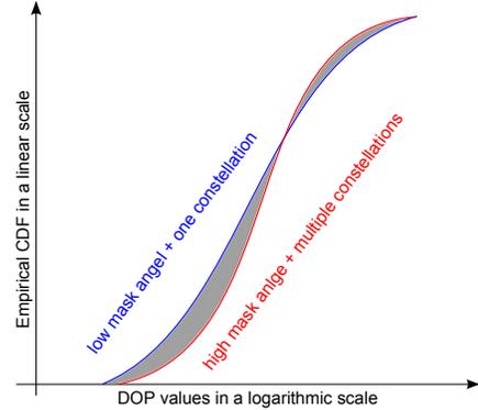
Fig. 2. The integral of relative difference between quantiles is equal to the area of the shaded region.
