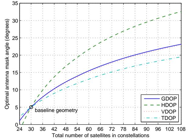
Fig. 5. The optimal antenna mask angle as a function of the total number of satellites for achieving GDOP, HDOP, VDOP, and TDOP of the baseline geometry.
