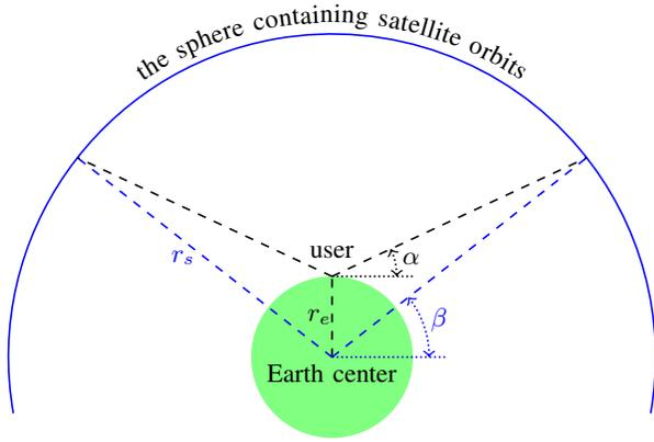
Fig. 3. Geometric method for calculating average number of satellites.  $\alpha$  is the antenna mask angle,  $r_s$  is the radius of satellite orbit, and  $r_e$  is the Earth radius.
