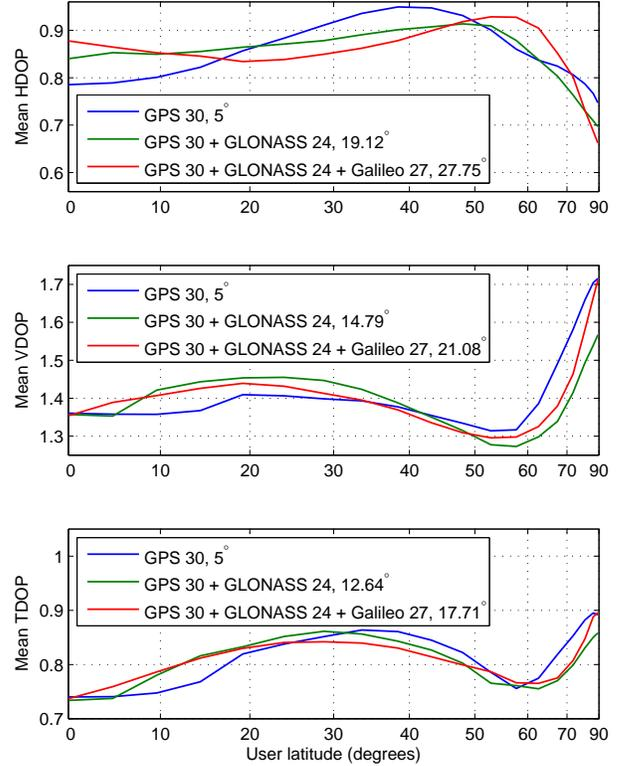
Fig. 9. Mean HDOP, VDOP, and TDOP values observed by users at different latitudes.
