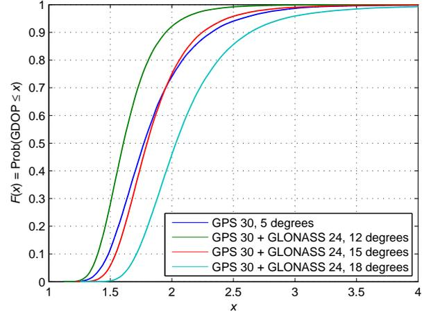
Fig. 1. Empirical CDF of GDOP values for a single constellation with a low mask angle versus that for multiple constellations with high mask angles. The CDF curve for multiple constellations cannot exactly match that for a single constellation.
