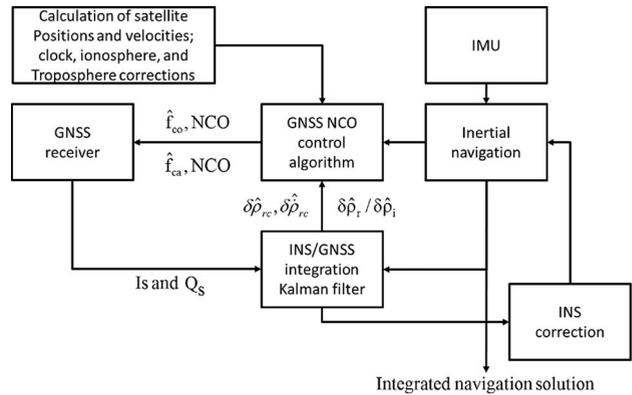
Fig. 3. Deep INS/GNSS integration architecture [18].
