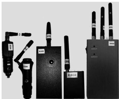
**Fig. 1.** GNSS jamming devices (PPDs) tested at Institute of Communication and Navigation, German Aerospace Center.
