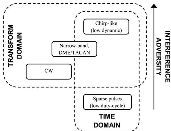
**Fig. 8. Guidelines on recommended mitigation operating domain for different interference sources.**
