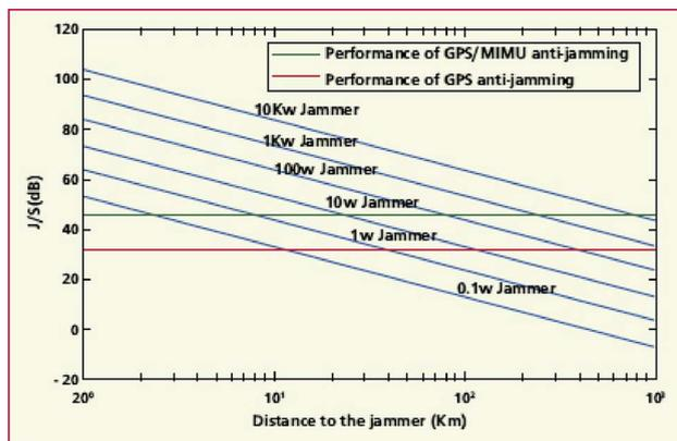
**Fig. 4. Performance of GPS/MIMU anti-jamming versus GPS anti-jamming [18].**
