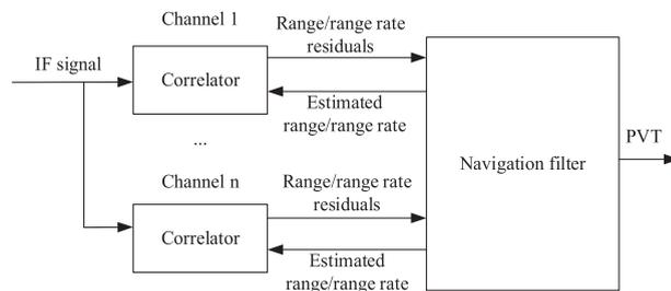
**Fig. 9. Vector tracking block diagram. Unlike classical scalar tracking, the tracking effort of individual GNSS channels are coupled through the shared receiver states of position, velocity, and time.**
