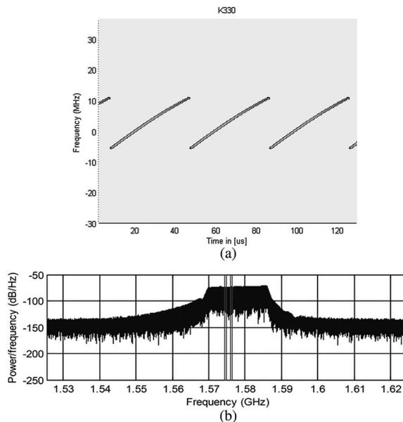
**Fig. 2.** Chirp-like PPD generated by a K330 Jammer: (a) Spectrogram. (b) Power spectral density.
