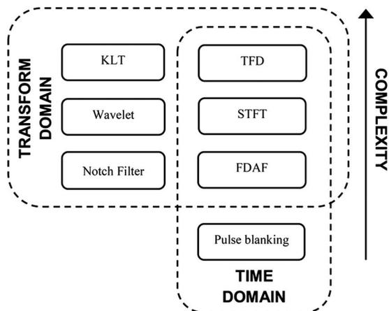
**Fig. 7. Classification and computational complexity of the interference mitigation techniques in time and transform domains examined in this section.**
