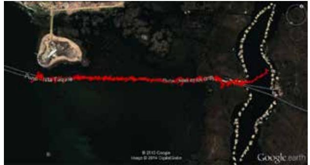
▲ **FIGURE 8** The trip back to Puno as determined by Receiver Y after cooperative scalar tracking and navigation computations. Compared to Figure 4, the navigation solutions are less noisy. Image courtesy of Google Earth and the GPS Visualizer.
